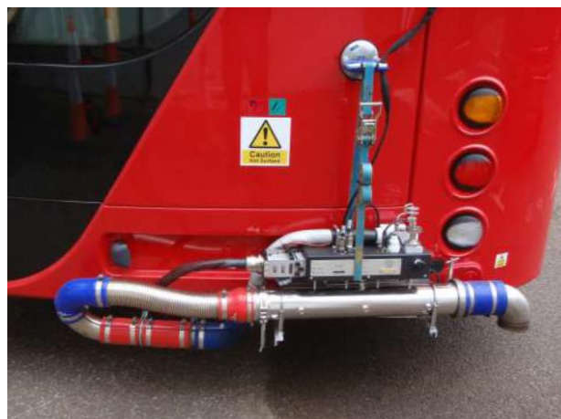
Figure 3: PEMS fitted to a bus exhaust system
