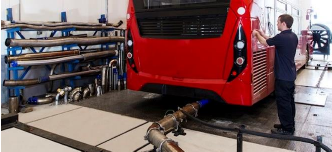
Figure 1: Bus chassis dynamometer testing
