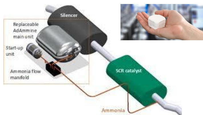
Figure 6: Ammonia Storage and Delivery System
