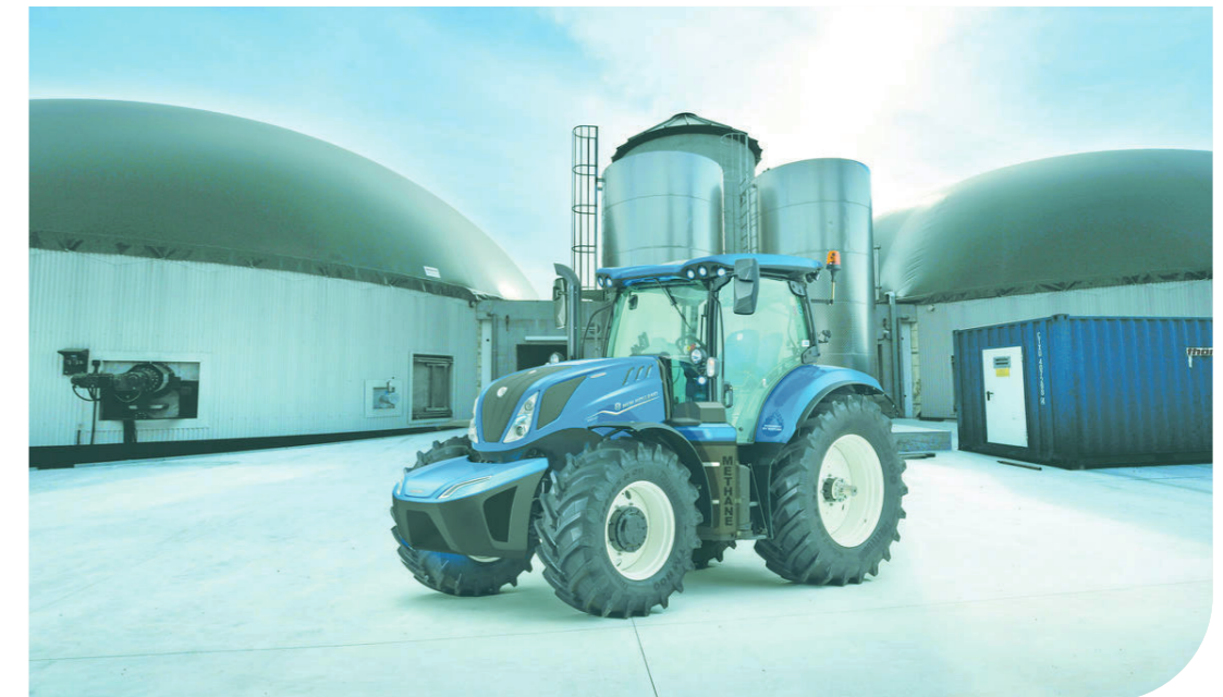
New Holland T6.180 Methane Power tractor showing additional gas storage at front
