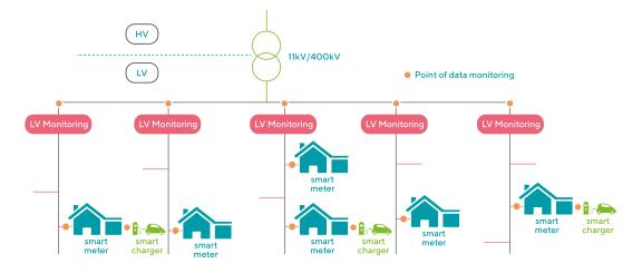
Figure 1 Different locations for monitoring the low voltage (LV) network
