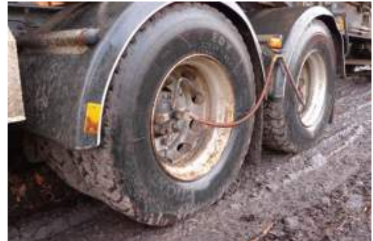
Automatic tyre pressure system
