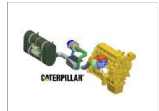
Picture: Caterpillar package layout – Brayton system 1)
