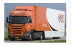
**Aerodynamic Fairings** Addition of trailer and cab fairings to help improve vehicle aerodynamics
