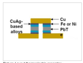
Picture: Layout thermoelectric generator, Ed Gundlach GM DEER 2008
