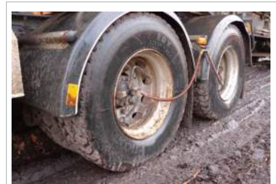
Picture: Automatic Tyre Pressure System (Freight Best Practice)
