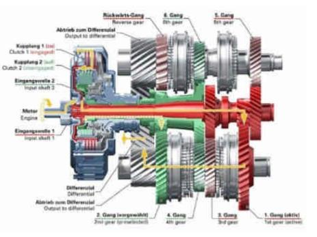
Audi DSG Dual Clutch Transmission Cutaway
