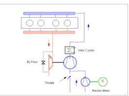
Picture: Electric assisted turbocharger Source: www.3k-warner.de
