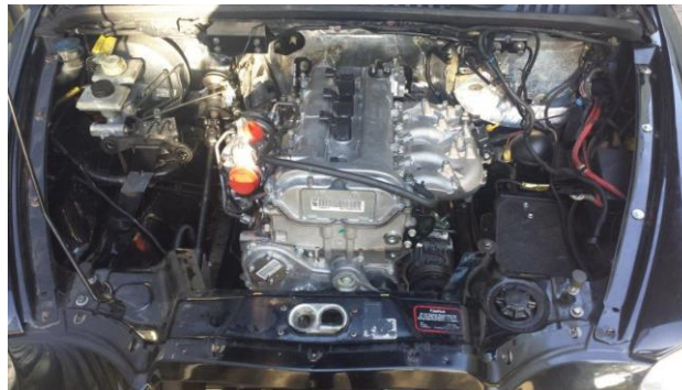
Spark ignition engine fitted in the taxi
