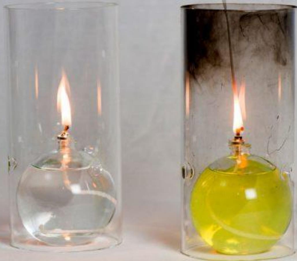
Left: Diesel made using Velocys process; right: diesel from filling station
