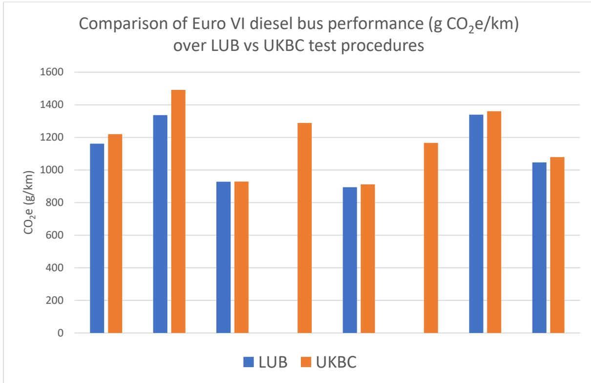
There was a small improvement in well-to-wheel CO<sub>2</sub>e emissions from Euro V to Euro VI when comparing like for like test results over the LUB cycle, despite the increased production of N<sub>2</sub>O from the conversion of NO<sub>x</sub> in the aftertreatment system. This demonstrates that manufacturers are continuing to improve diesel vehicle efficiency through improved driveline and new energy management systems alongside light weighting strategies.
