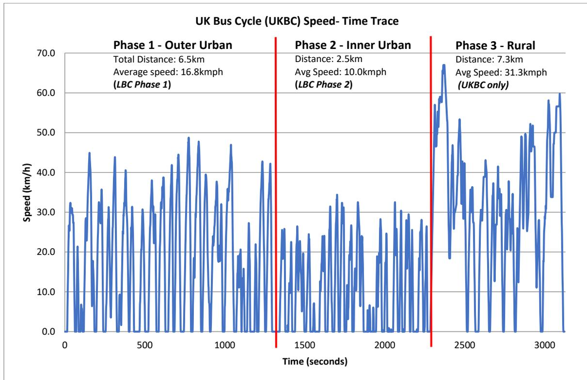
A key objective in the formation of the UKBC was to ensure the test processes align with those undertaken by Transport for London (TfL). As a result, TfL's new **London Bus Cycle** (LBC), previously the MLTB cycle (route 159), can be extracted directly from the UKBC by the test house, for all propulsion types.
