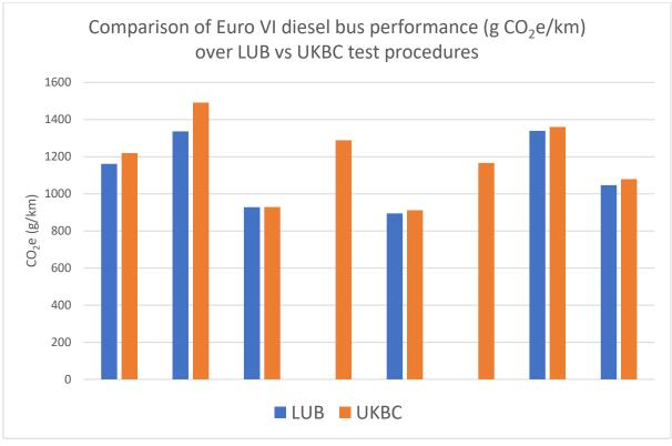
There was a small improvement in well-to-wheel  $CO_2e$  emissions from Euro V to Euro VI when comparing like for like test results over the LUB cycle, despite the increased production of  $N_2O$  from the conversion of  $NO_x$  in the aftertreatment system. This demonstrates that manufacturers are continuing to improve diesel vehicle efficiency through improved driveline and new energy management systems alongside light weighting strategies.
