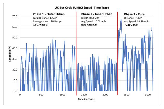
A key objective in the formation of the UKBC was to ensure the test processes align with those undertaken by Transport for London (TfL). As a result, TfL's new **London Bus Cycle** (LBC), previously the MLTB cycle (route 159), can be extracted directly from the UKBC by the test house, for all propulsion types.
